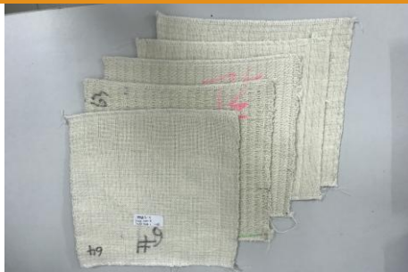
Nickel iron fiber/cotton absorbing woven fabric
