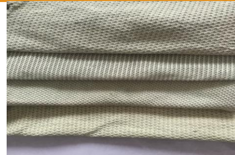
Nickel iron fiber/cotton absorbing knitted fabric
